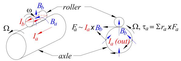
The magnitude of the torque scales (in Gaussian units) as  $\sigma \Omega I_a^2/c^4$  where c is the speed of light.
