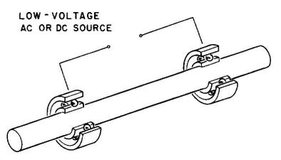
Note that this motor is not self-starting in general; the axle must typically be given an initial angular velocity, of either handedness, after which the motor can sustain rotary motion, if the current (AC or DC!) is large enough.
